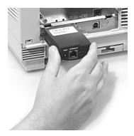
3. Secure the OkiLAN 6020e with the wire clips on the printer's connector.
